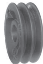
133508 Servicing VG-986, -921, Ikarus Cargo 110541, 110543, 110544 O.D. 105 mm, Bore 30 mm Double, B-type belt
