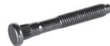
231868 Std pkg 10 M5 x 40 mm KNURL O.D. 5.5 mm Screw for S.R.E. bracket
