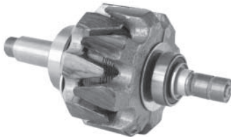
134471 Servicing VG-986, -921, Ikarus Cargo 110541, 110543, 110544 24 V. L. 258.3 mm, O.D. 126 mm, Shaft 30 mm
