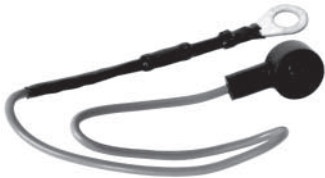
232761 Servicing 27SI/200 150 Ohm. Resistor, connects from battery terminal to pin-type R-terminal for faster cut-in speed
